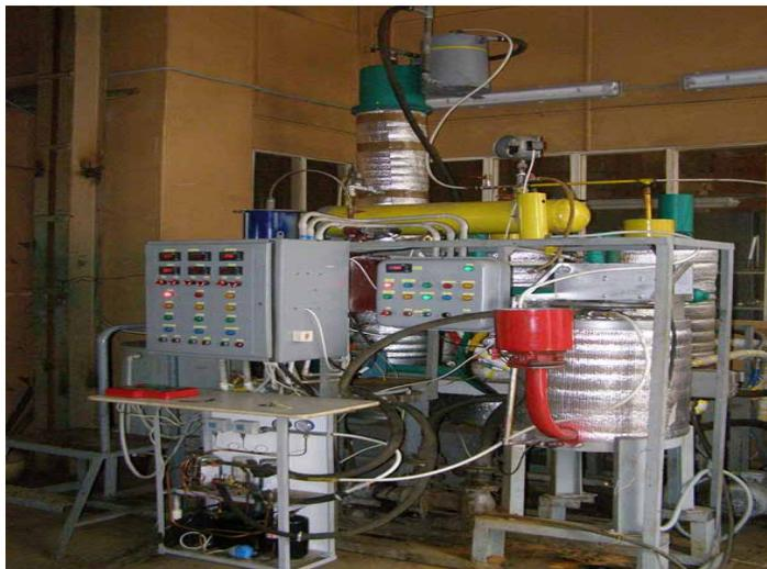
Heat pump: R717 refrigerant; compressor KF 130, compressor capacity 1 kW; evaporator, condenser and superheater - plate heat exchangers M12-50 GL GL.
